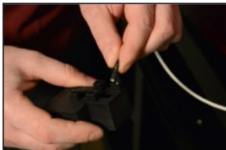
2 - Reconnect the ignition electrode cable to the igniter assembly, taking care not to damage the cable or the connection.
