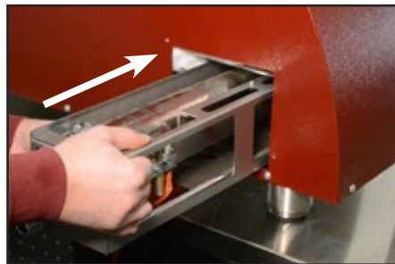
4 - Fully insert the burner. Position the burner so it fits into the guide rail. Slide the burner along the guide rail until it reaches the front stop position. Make sure the ignition electrode cable does not become tangled.
