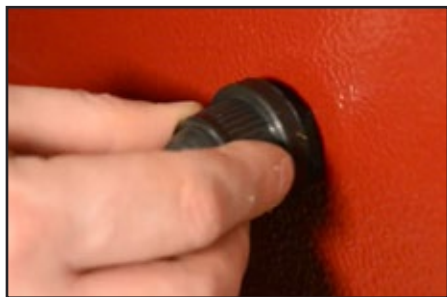
3 - Insert the igniter assembly and screw in the igniter.
