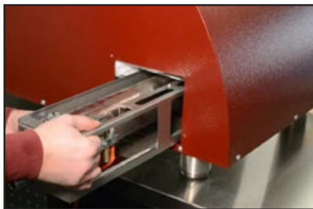
4 - Fully insert the burner. Position the burner so it fits into the guide rail.
